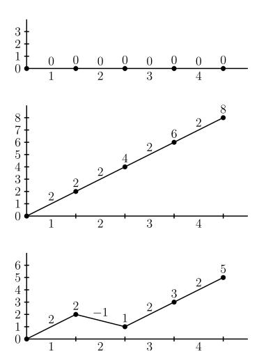
Views of the track before and after each reconfiguration. The x axis denotes the rail number. The y axis and the numbers over points denote elevation. The numbers over segments denote elevation changes.
